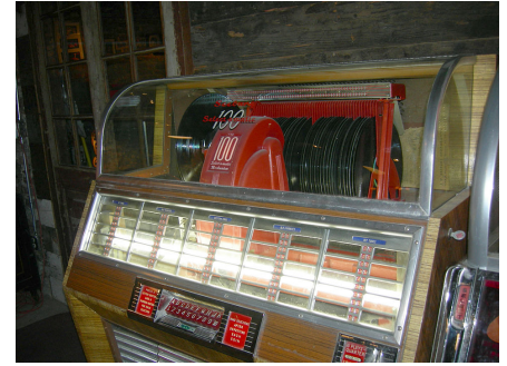
A jukebox. At the top are records; at the bottom are buttons to select which record to play.
